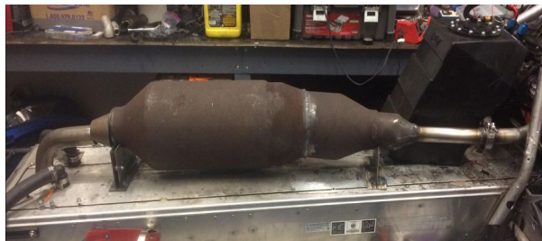
Figure 8: Catalyst and Diesel Particulate Filter
