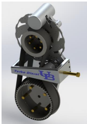
Figure 15. Belt Drive Assembly Designed in SolidWorks
