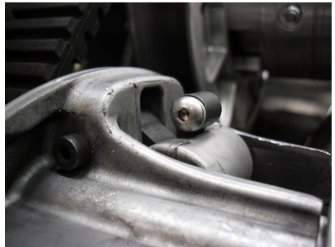
Figure 3: Adjustable Clutch Weight in Drive Clutch
