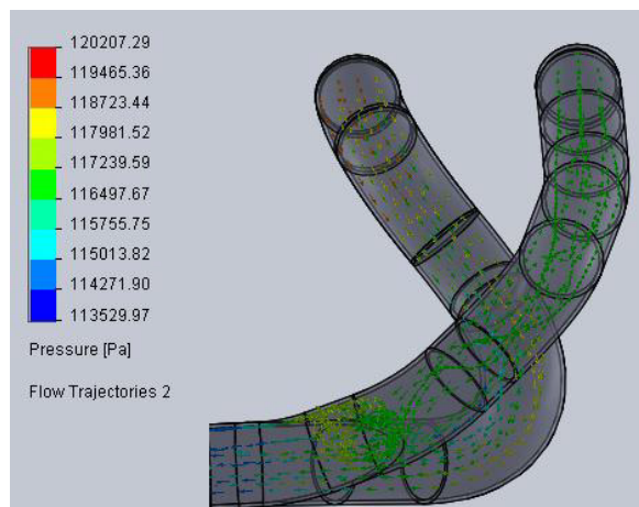
Figure 5 - Header Pressure Profile when MAG Cylinder is on Exhaust Stroke
