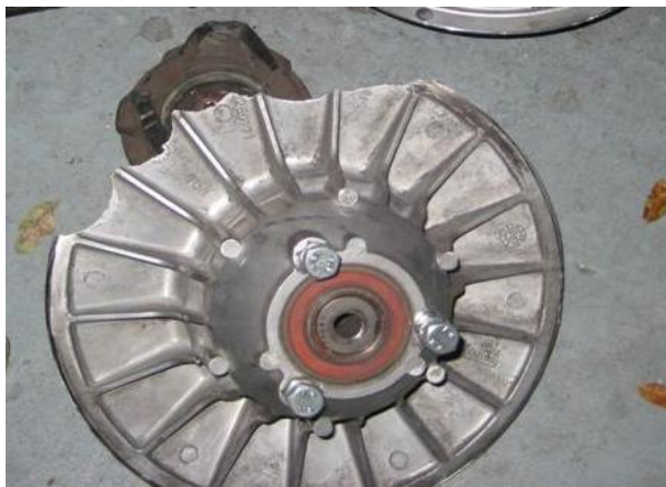
Figure 12: Destroyed driven clutch
