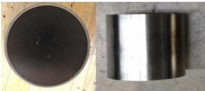
Figure 7. A top and side view of the 3 way catalytic converter.
