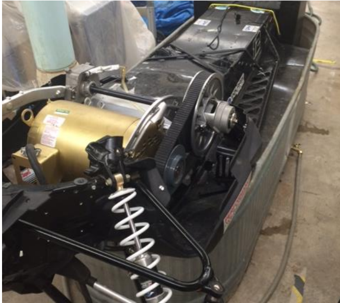
Figure 20. The chassis dyno with a 10 horsepower motor and the track suspended in water.
