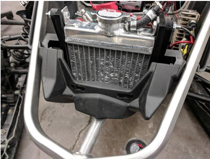
Figure 4. The aluminum radiator mounted in the nosecone of the snowmobile.
