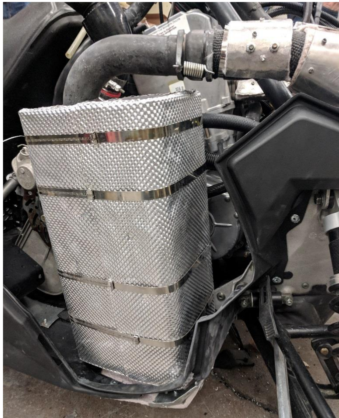
Figure 22. The muffler mounted in the snowmobile, with heat shields.
