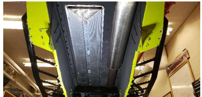
Figure 15. Rear-exiting exhaust (resonator) and tunnel cooler mounted in newly designed tunnel
