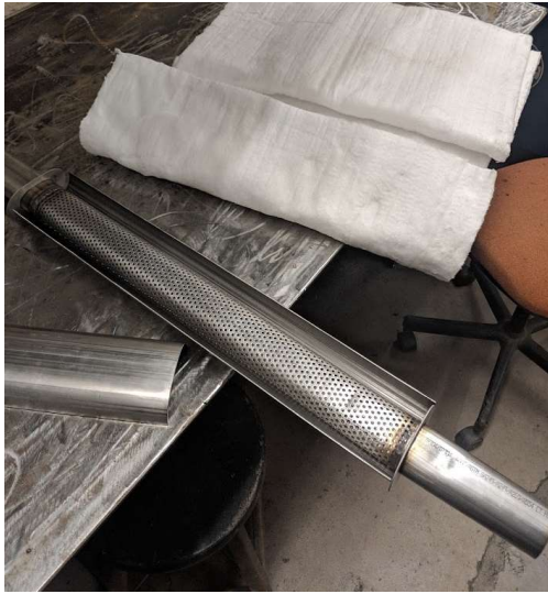
Figure 19. Resonator tube prior to final assembly
