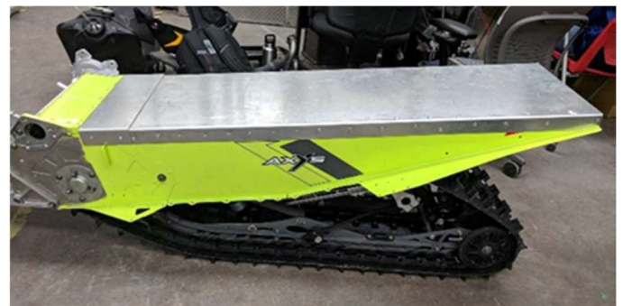
Figure 25. Tunnel modification on the 2019 Polaris Indy XC 129
