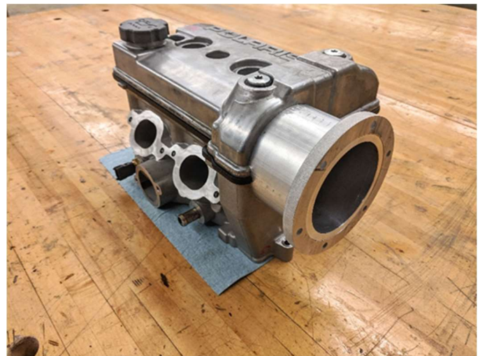
Figure 6. Camshaft phaser and solenoid housing installed on an adapted ProStar 1000 cylinder head
