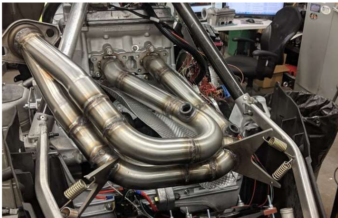
Figure 20. Tuned exhaust header mounted in the snowmobile's bulkhead
