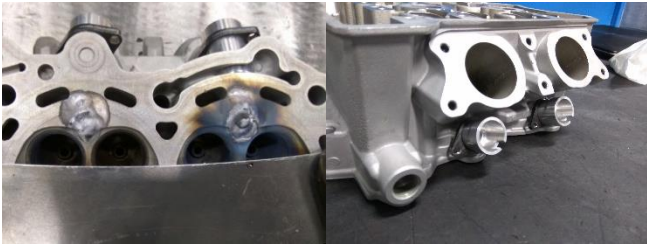
Figure 3. Welded injector holder tips and final head assembly
