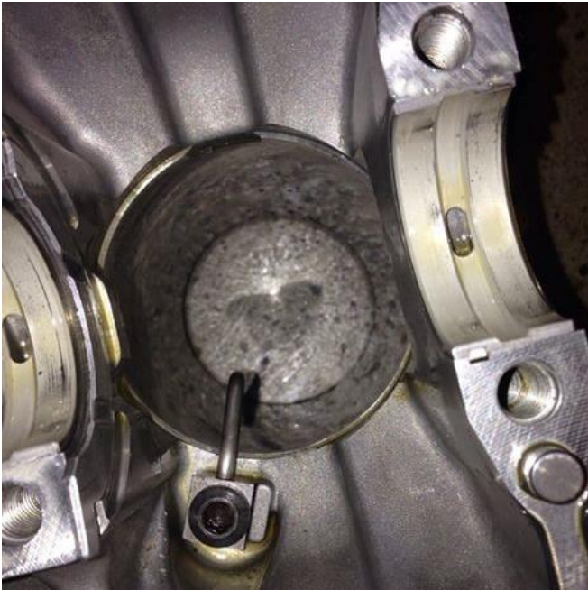
Figure 6. Piston Coolers Installed
