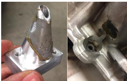
Figure 1. Previous version of the failed injector holder and cylinder head
