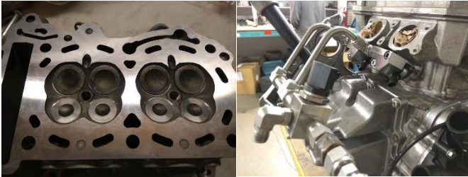
Figure 4. Milled cylinder head face and complete head assembly
