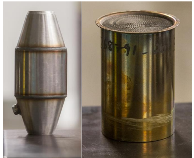
Figure 4. DPF and DOC Used with our Kohler Engine
