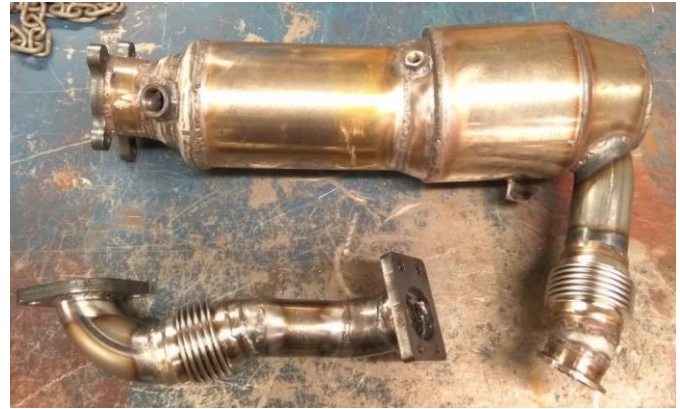
Figure 2. New Exhaust System
