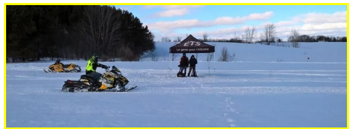
Figure 12. Sound Test Performed Outside as per the Competition's Rules
