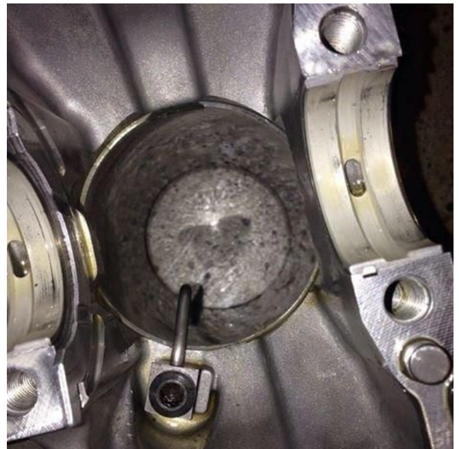
Figure 5. Piston Coolers Installed
