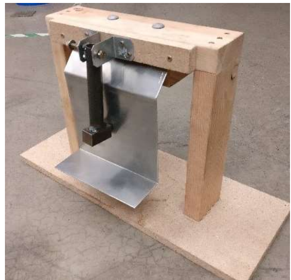
Figure 13. Tunnel resonance test apparatus.
