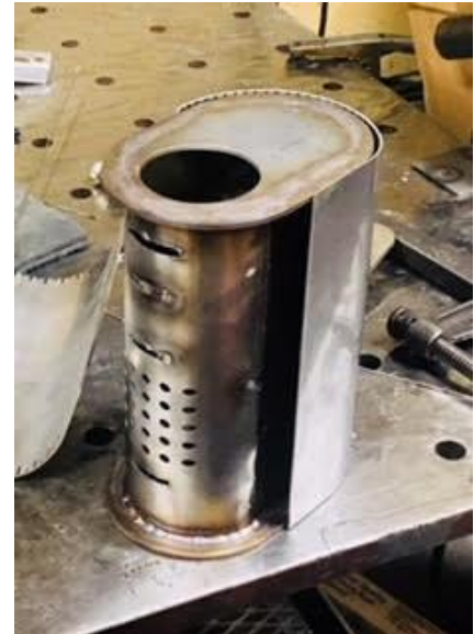
Figure 10: Final Muffler Design - Dual Wall Cutaway
