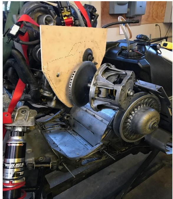
Figure 1: Shows use of wood to attain rough shape and size measurements of PTO side engine support.
