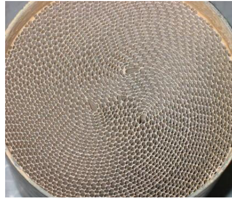
Figure 17. Catalytic Converter Cross Sectional View.
