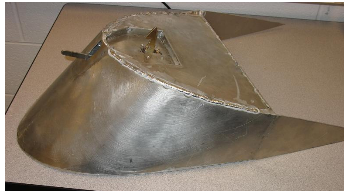
Figure 3. Custom Fuel Tank.
