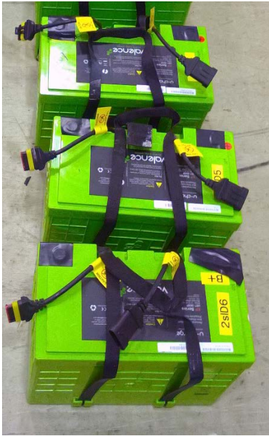
Figure 9. Valence U-Charge@ U27-36XP modules before installation to battery container.
