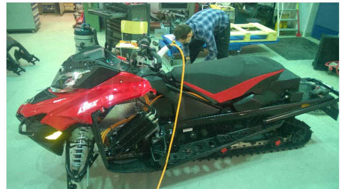
Figure 2. Our eSled built on Lynx Adventure 2016 LX 600 ACE chassis having final preparations before CSC 2016.
