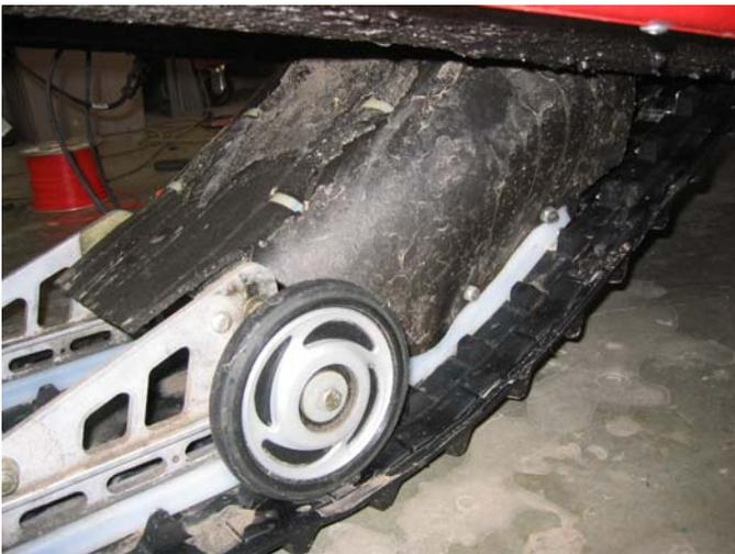
**Figure 16:** Drive paddle sound dampener installed on front suspension arm.
