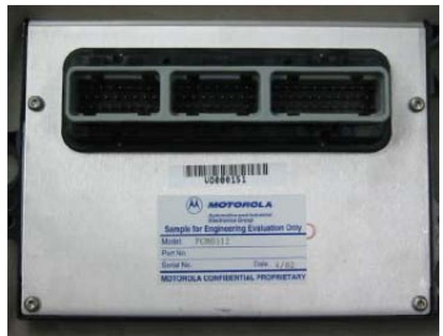
**Figure 6:** Picture of the Motorola MPC555 powertrain control module.
