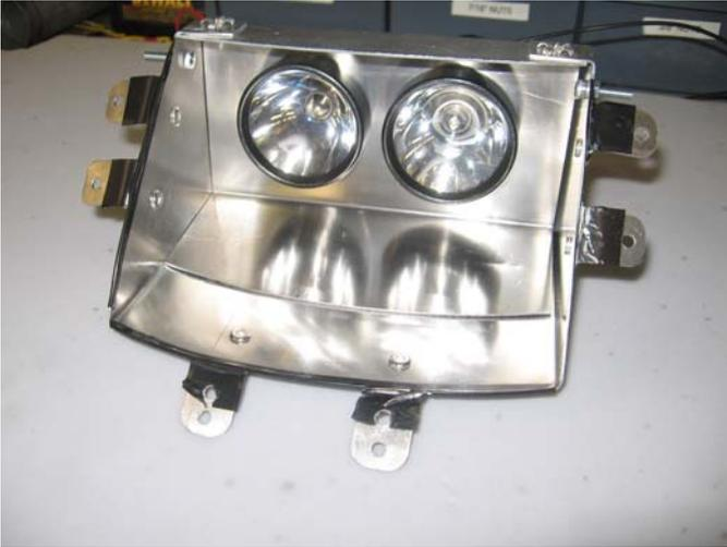
**Figure 22:** Dual LED headlight assembly before installation.
