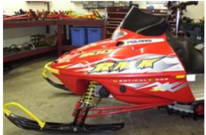
**Figure 24:** Picture of the lightweight front suspension being utilized by Wisconsin.
