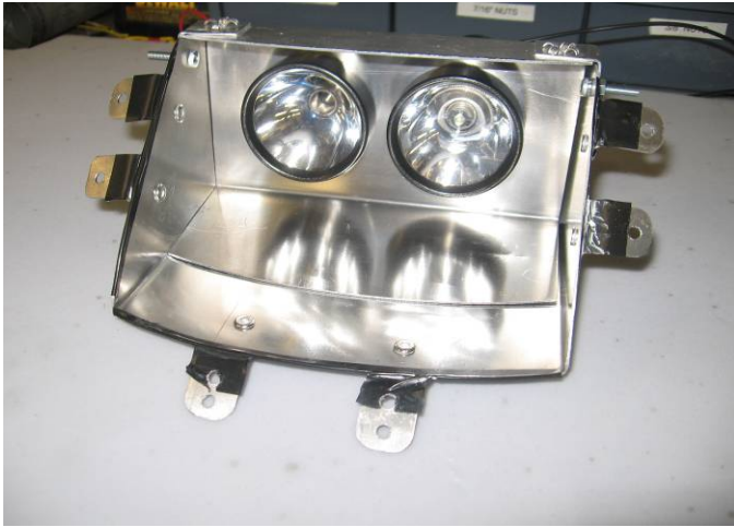
Figure 24: Pictures of the dual LED headlight assembly before installation.
