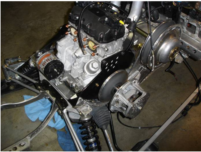
Figure 4: Picture of the clutch-side engine mounting bracket during fabrication phase.
