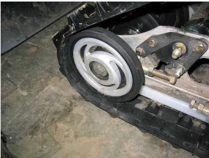
Figure 17: Picture of the Arctic Cat Silent Track installed in the Bucky 750 FX.
