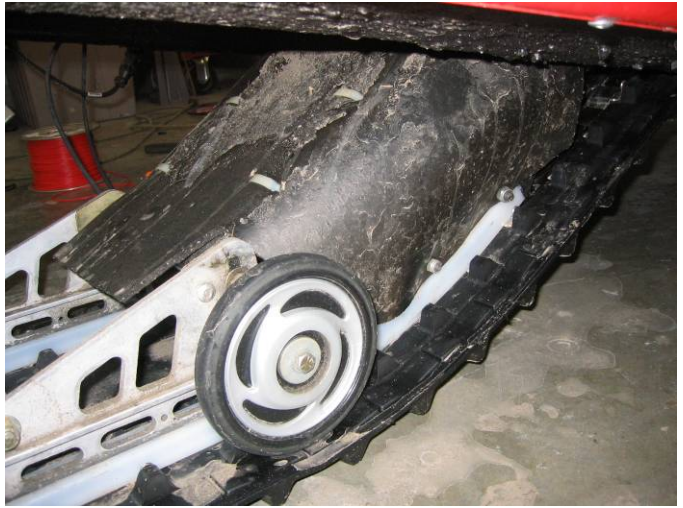
Figure 18: Picture of the drive paddle sound dampener installed on front suspension arm.
