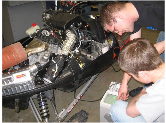
Figure 9: Picture of the students huddling around an oscilloscope calibrating the new E85 injectors.
