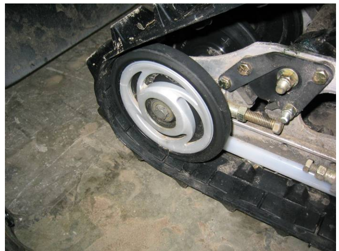
Figure 21: Picture of the Arctic Cat Silent Track installed in the Bucky CFS.
