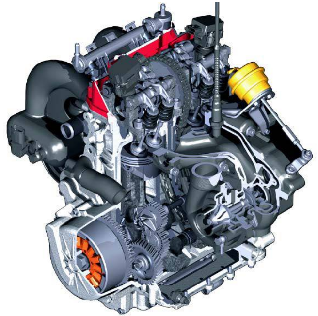
Figure 4: Model of the PWC version of the Weber AG MPE 750 engine.
