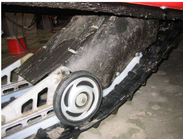
Figure 22: Picture of the drive paddle sound dampener installed on front suspension arm.
