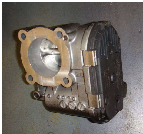
Figure 6: Picture of the Bosch electronic throttle body utilized on Polaris MSX personal watercrafts.
