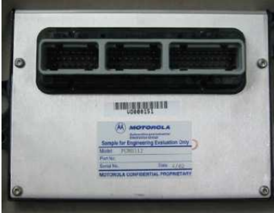
Figure 3: Picture of the Motorola MPC555 powertrain control module which is used as the engine control module in the Bucky CFS.
