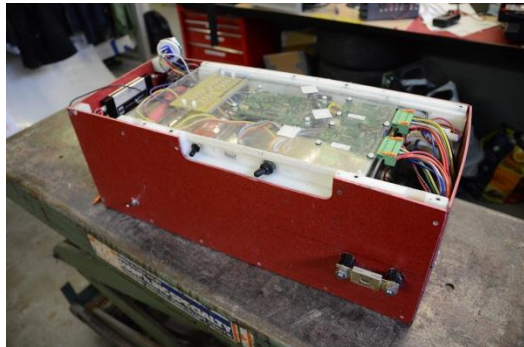
Figure 2 – 2012 Battery box design
