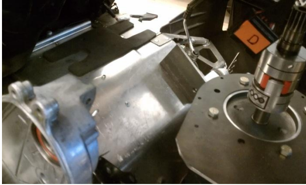
Figure 10 - Motor Mounting Point Before adding Damplifier Pad
