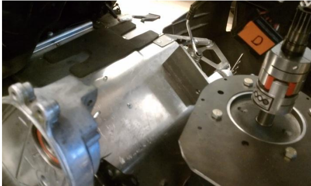
Figure 10 - Motor Mounting Point Before adding Damplifier Pad
