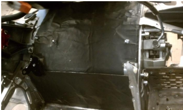
Figure 11 - Motor Mounting Point after adding Damplifier pads
