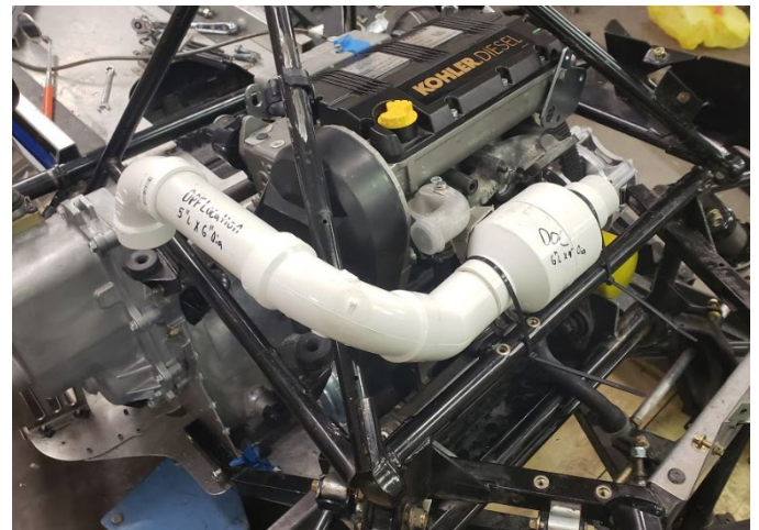
Figure 4: Prototype mock-up of aftertreatment system
