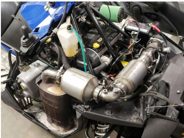
Figure 6: Final exhaust and aftertreatment mock-up
