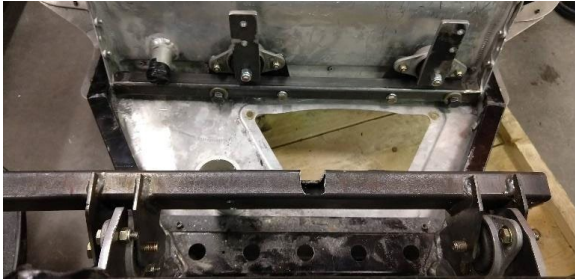
Figure 2: Assembled engine mount components in the snowmobile.
