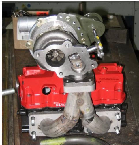
Figure 4: IHI RHB-5 Turbocharger implemented on the 2007 MTU Entry
