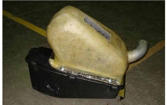
Figure 23: MTU Custom Air-box Enclosure
