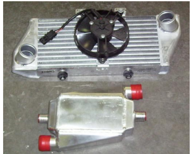
Figure 5: Stock Intercooler (top) Compared to MTU's Bell Intercooler (bottom)
