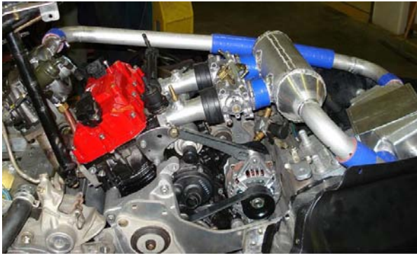
Figure 3: MTU Custom Designed and Fabricated Intake System
