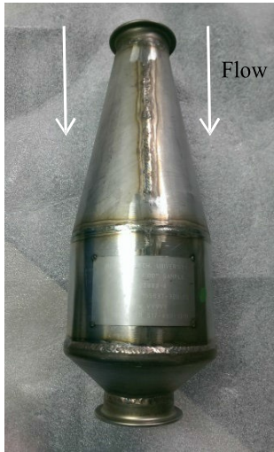
Figure 8: The catalytic converter that will be used in the MTU exhaust system that will reduce the levels of UHC, NO x and CO
