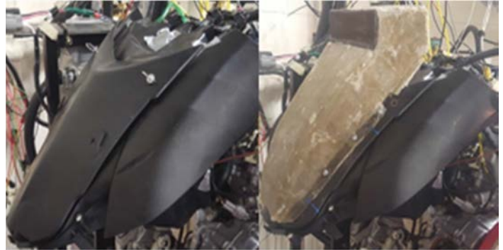
Figure 17: Original vs. prototype air box intake
