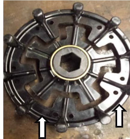
Figure 19: MTU custom driver before isolation rubber installed. Arrows depict the slots cut to be filled with the isolation rubber.
