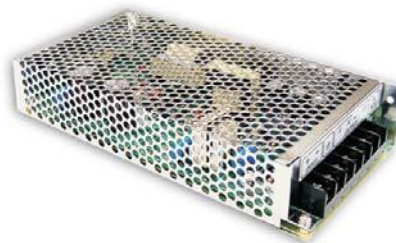
Figure 5: SD-150D-12 DC to DC Converter [4]
