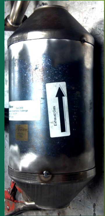
Emitec PM METALIT Partial Flow DPF (D=4.65" x L=6.5")
