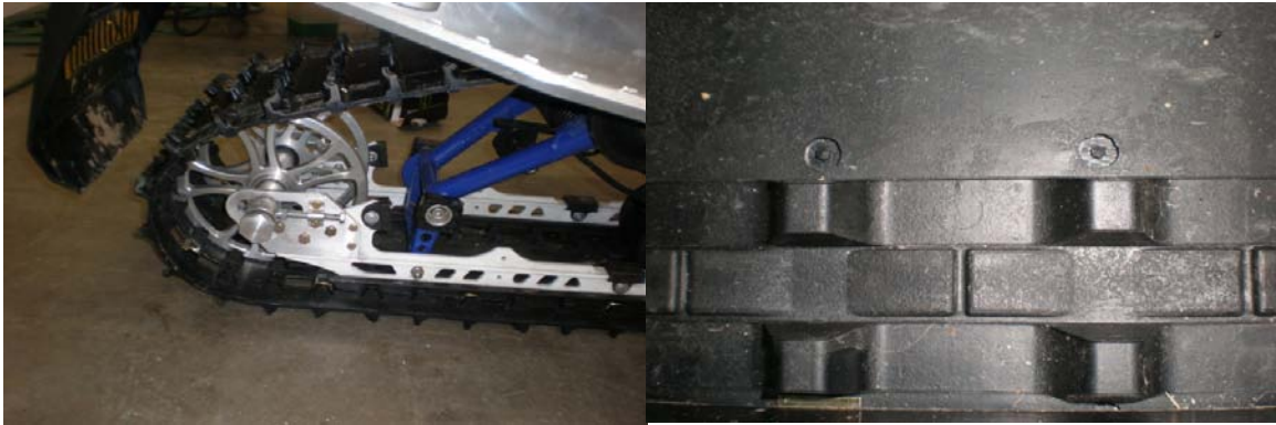
Figure 7: Ten inch CNC wheels with 128 inch track (left), quiet track ramps on the 13.5"x1"x128" track (right)
