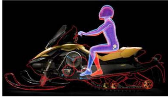
Figure 5: Red outline shows the riding position and layout of the Rev, blue outline shows the Rev-XP [17].
