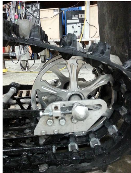
Figure 3: Ten inch idler wheels with 136 inch track
