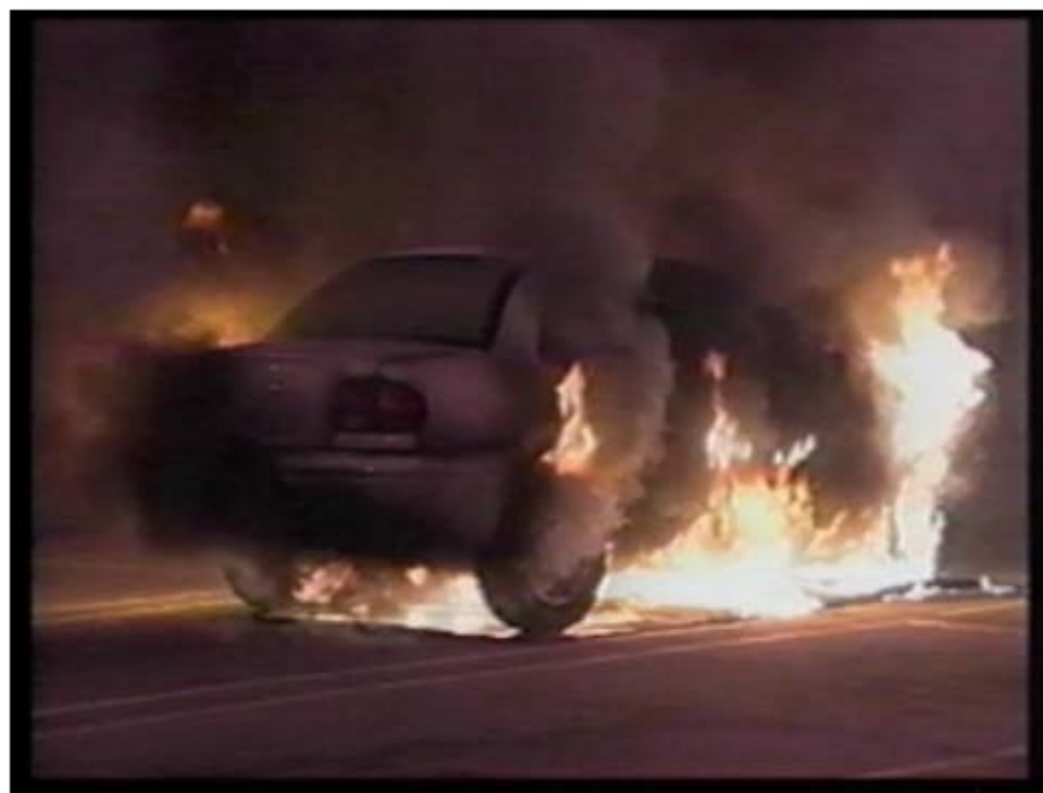
Photo 5 - Time: 2 min, 20 sec - Frame prior to interior deflagration.
