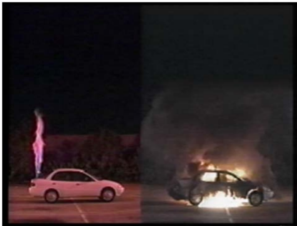
Photo 3 - Time: 1 min, 0 sec - Hydrogen flow is subsiding, view of gasoline vehicle begins to enlarge
