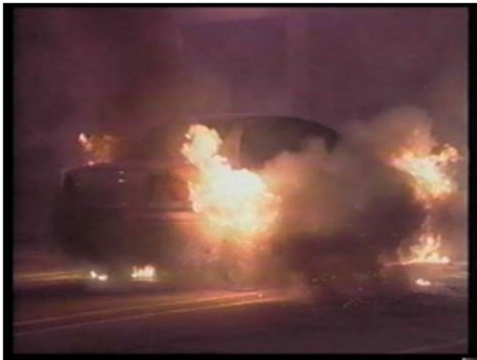
Photo 8 - Time: 2 min, 40 sec - Driver's side rear tire rupture sends debris out the passenger side of the vehicle.
