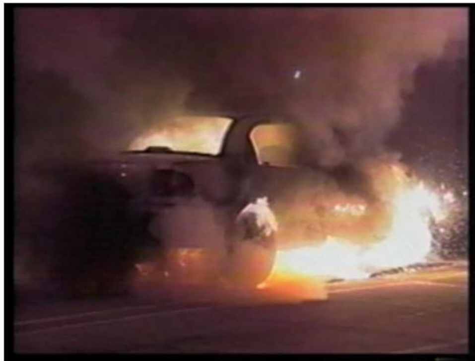
Photo 6 - Time: 2 min, 20 sec - Deflagration in the interior, following frame shows flames exiting around edges of trunk lid.
