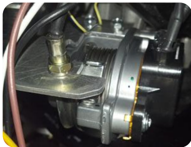
Figure 14: Acura TL FPS. Note the cable actuation. This is a somewhat unique design
