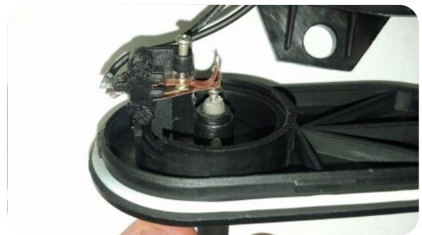
Figure 9: Internal vacuum regulator
