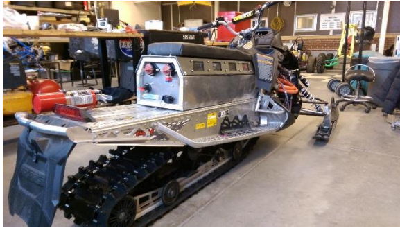
Figure 6: The battery box also serves as the seat of the snowmobile.
