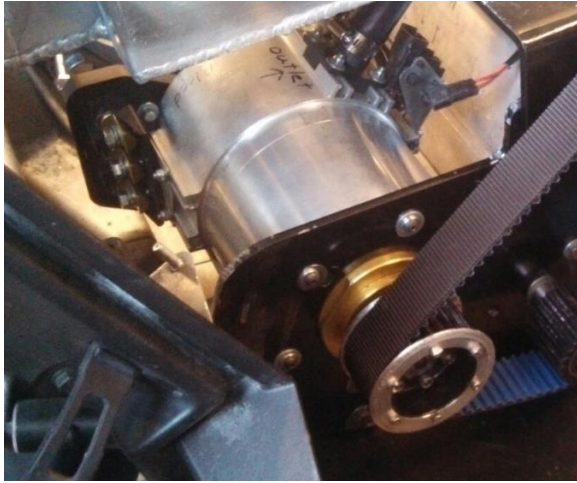
Figure 14: Liquid cooled Parker/Brammo permanent magnet AC motor.
