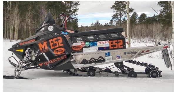
Figure 17: The seat is comfortable and provides an ergonomically correct riding position. ProTaper handle bars offer both stand up and sit down comfort.
