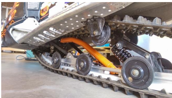
Figure 9: New suspension to improve load and roll handling capabilities. Note the
