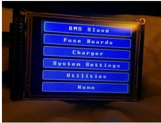
Figure 3: BMS system utilities screen allows accessing and changing many parameters
