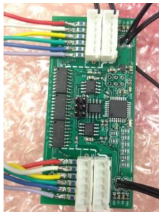
Figure 4: Fully isolated fuse monitoring solution detects possible open fuses and measures temperature of every cell in the pack
