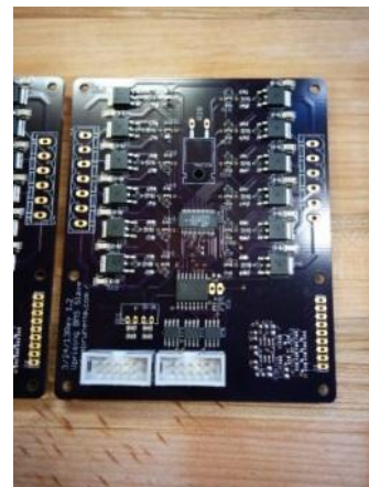
Figure 2: Team-built Battery Monitoring board based on LTC6803 chip
