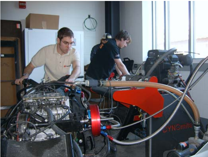
Figure 5: Dyno testing using Land and Sea Dynamite
