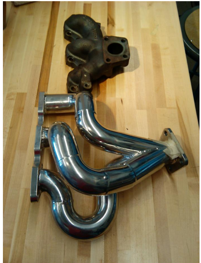
Figure 7: Stock exhaust manifold (top) versus redesigned manifold (bottom).
