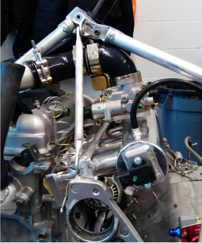
Figure 4: Redesigned manifold attached to the engine, in the chassis.
