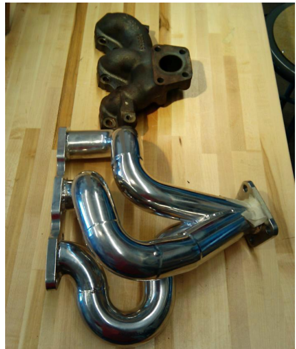
Figure 5: Stock manifold (top) vs equal-length exhaust header (bottom)
